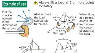
When lifting a long load, lift at 4 or more points, and use a balance whenever possible. (for safe operation, the lifting angle of the sling ropes must be kept within the specified angles.)
