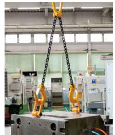
Seating face contact is essential for the eye bolt, but the ring direction is inconsistent...
