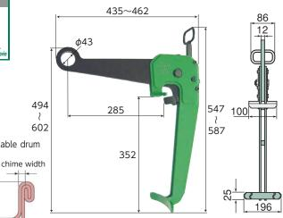
JIS Z1601 type : H class and M class (with 600mm $\phi$  lid) and drum cans with lid of 500 to 700mm in diameter, with chime thickness of 2 to 3.5mm and chime height of 22 to 28mm (lifting is vertical only for  $600mm\phi$  lid).
