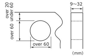
⚠ The applicable road plate thickness and hole dimensions shall be within the ranges of the drawing and the chart.
