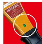
This is an overload sensing device, which displays an overload indication (green -> red) in the window of the lever at the same time that the lever tip (handle grip portion) bends in overload working.
