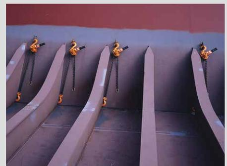
Shape is cut out with special tip so it can hook on to the edge of steel plate making it suitable for certain shipbuilding or plate working applications. (Not suitable for general load holding, taking-up, or lifting applications – use standard hook instead).
