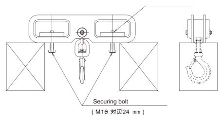
(4) Insert the forks into holes for the forks of the fork lift and position them to be fixed.(When inserting the forks, take care not to collide with the lifting clamp)Next, raise the forks up in order to easily tighten the securing bolts.
