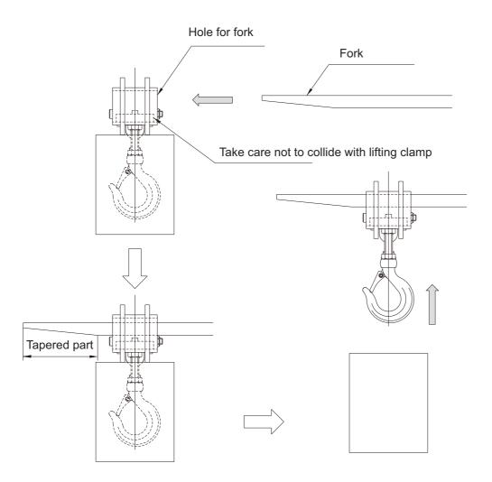
(5) Tighten the lifting clamp and forks of the fork lift by securing bolts (The angle of the forks of the fork lift must be horizontal at this time) Never use when the fork of the fork lift is not horizontal.
