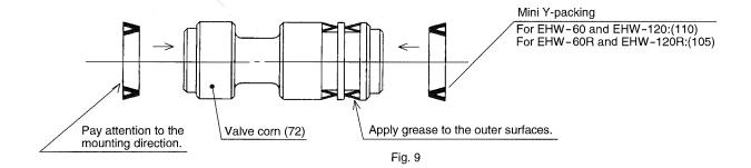
④ A jig is required when installing Valve cone (72). (See Fig. 10.)
