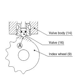
Small recess (a) on Index wheel (9) should be in contact with the tip of Valve (16).
