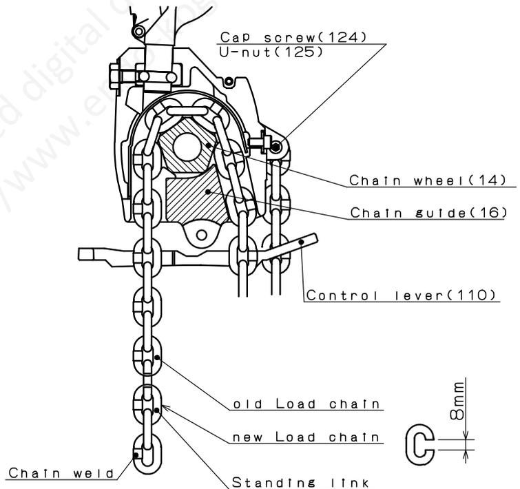
Slowly operate the hoist in the lifting direction, feeding out old Load chain, leaving new Load chain on the Chain wheel(14).
