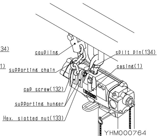
Fig.4 example of using supporting chain
