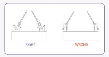
Make sure that the chain shackle is supporting the load correctly, along the axis of the shackle body centerline.
