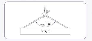
When a shackle is used to connect two slings to the hook of a lifting device, Anchor shackle must be assembled with the slings in the shackles body and the hook engaged with the shackle pin. The angle between the slings should not exceed 120°.
